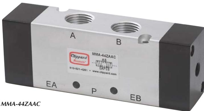
Maxematic® four-way 3-position double air pilot valves with closed center, pressure center or exhaust center spools are available in #10-32 thread to 1/2" NPT port sizes. These air piloted valves have 1/8" NPT external pilot ports.
